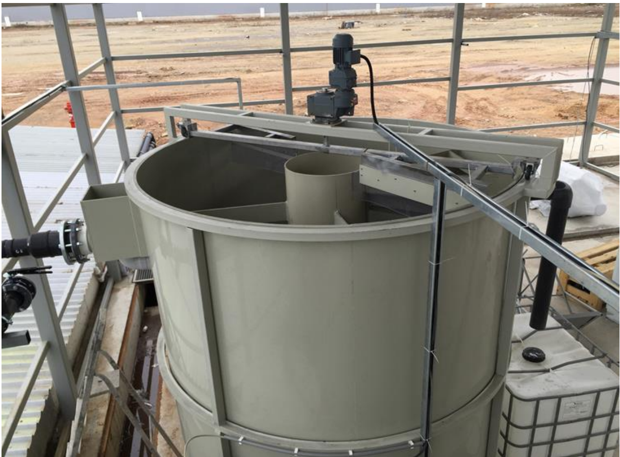
DAF (Dissolved Air Flotation ) System For Removed to Rolling Mill Oil by Water
