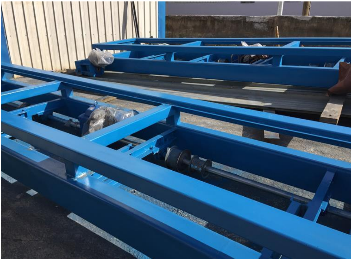
Settling Basin Scrapper Bridges
