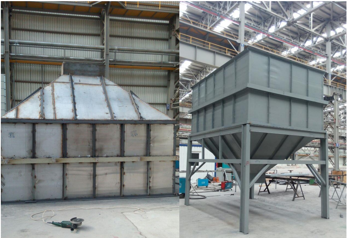
Sludge Thickener Tanks
